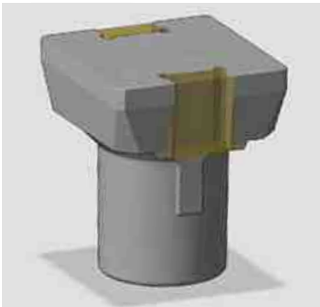
FIGURE 1: Steel piling hammer casting model
